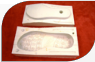
3.Molde en colada de silicona / Mould in straining silicone.
